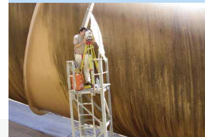
Measuring method with theodolite
